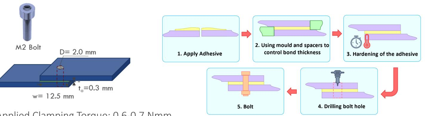
Applied Clamping Torque: 0.6-0.7 Nmm
