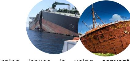
issues in using conventional metallic Concerning materials: lack of weight/fuel efficiency, low fatigue resistance, and electrolytic corrosion
